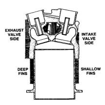
**cylinder barrel** — That portion of the cylinder or a reciprocating engine in which the piston moves up and down.
