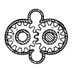
is carried around the housing of the rotating gears to the discharge side of the pump, the gear teeth mesh, and the fluid is forced out of the outlet side of the pump.
