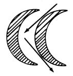
**impulse-reaction turbine** — A stator vane and rotor blade arrangement whereby the base area is an impulse design and the tip is a reaction design. This design is common to flight engines.
