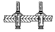
**grip range** — The difference between the maximum and minimum thickness of material that may be joined by a fastener.
