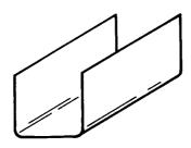
**channel iron** – Extruded steel either extruded or bent into a U-shape.
