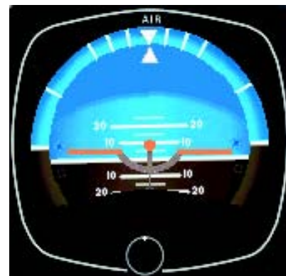
Figure 5-5. Pitch correction for level flight, two-bar width.
