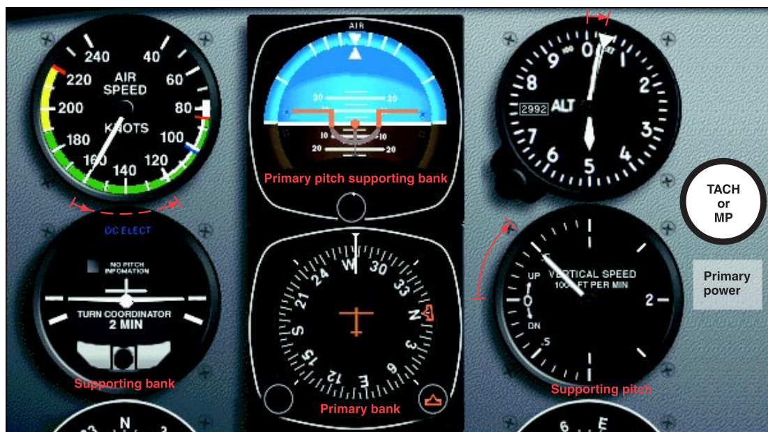
Figure 5-25. Climb entry for constant-airspeed climb.
