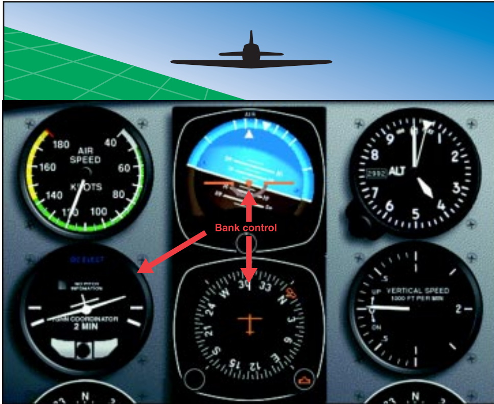
Figure 5-16. Instruments used for bank control.
