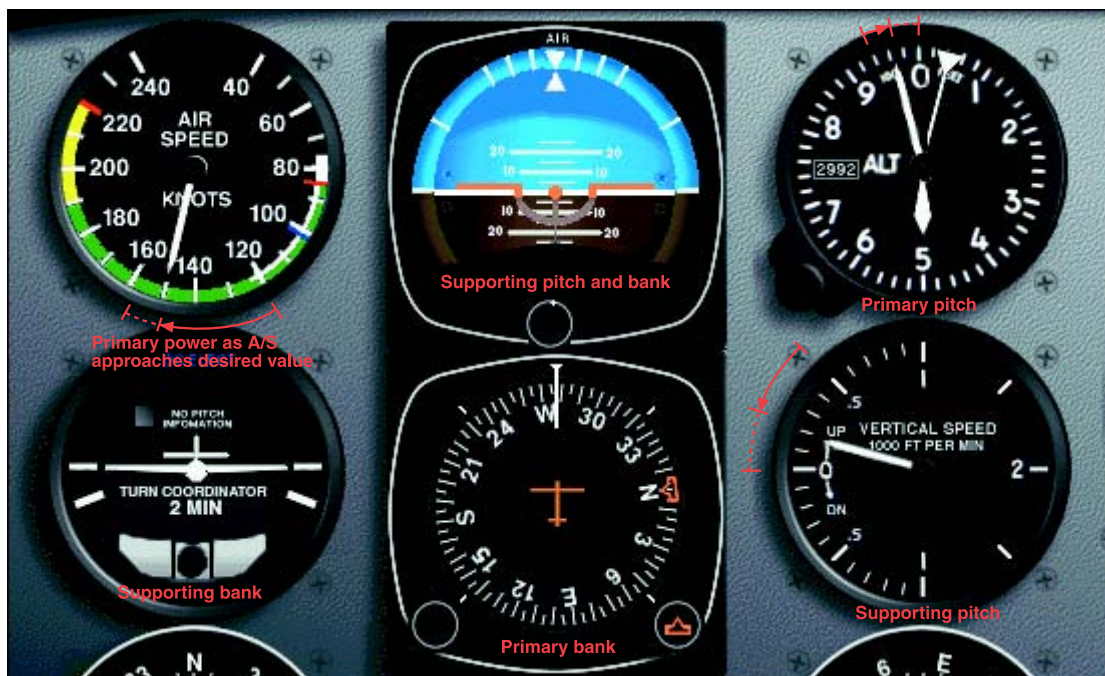
Figure 5-29. Level-off at cruising speed.
