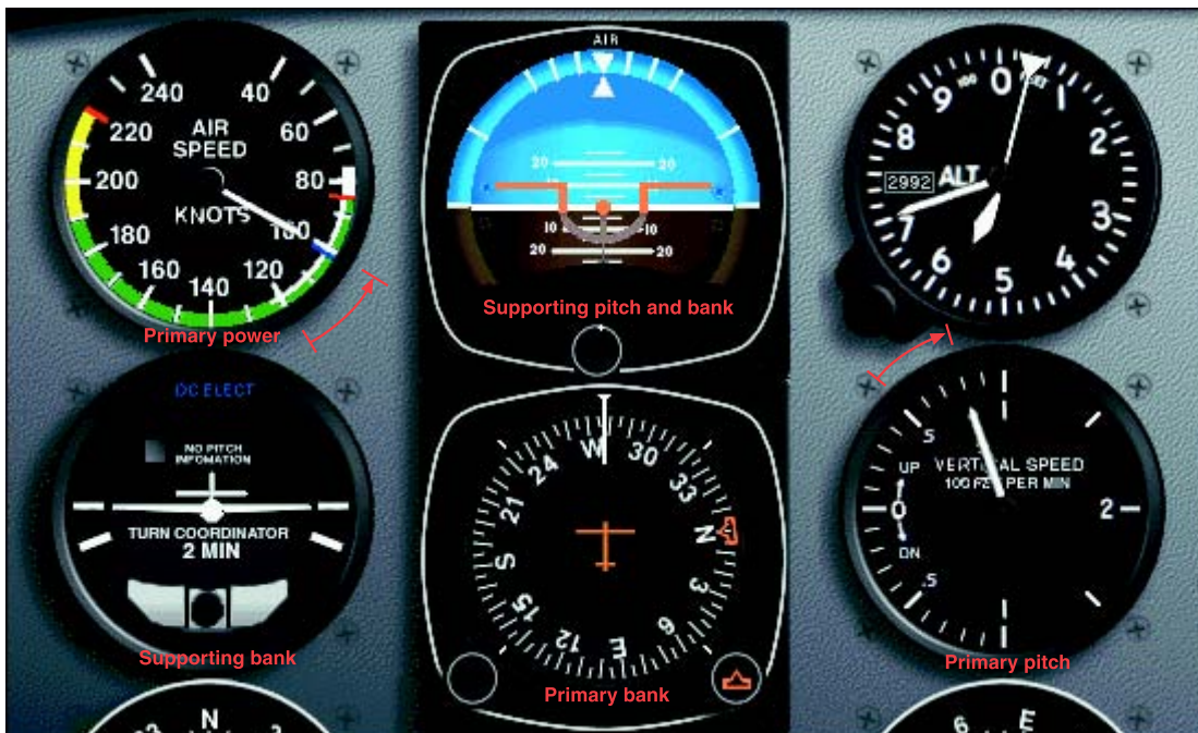
Figure 5-28. Airspeed low and vertical speed high—reduce pitch.
