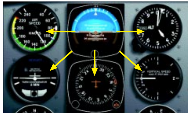
Figure 4-3. Selected radial cross-check pattern.
