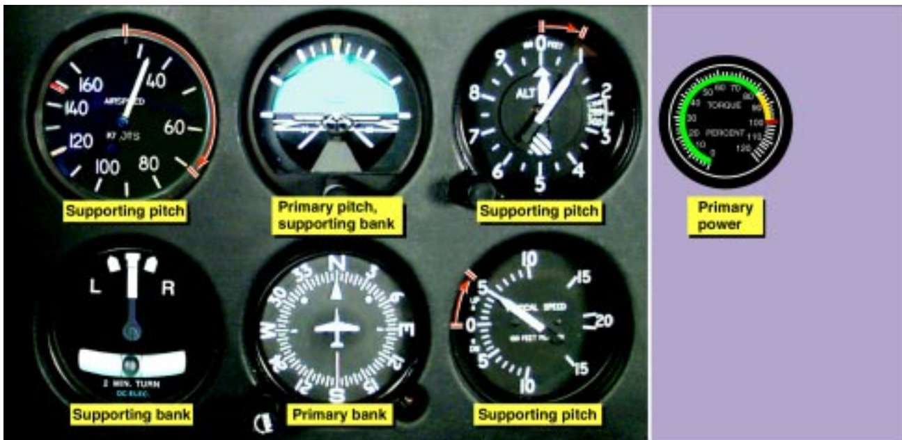
Figure 6-13. Flight instrument indications during an instrument takeoff.
