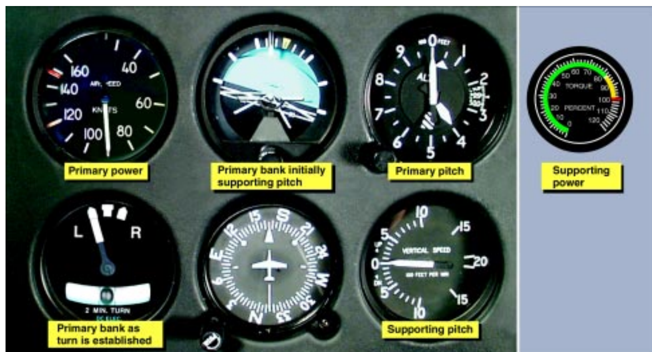
Figure 6-11. Flight instrument indications for a standard-rate turn to the left.
