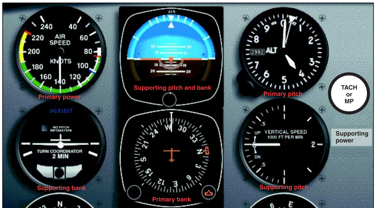
Figure 5-22. Straight-and-level flight (normal cruising speed).
