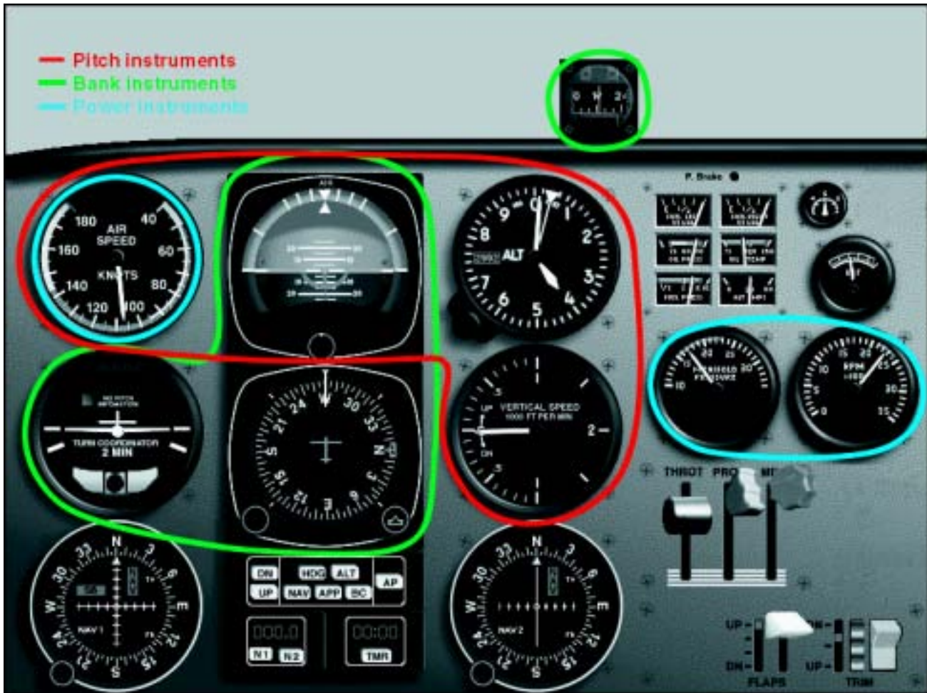
Figure 4-2. Primary/Supporting cross-check method.
