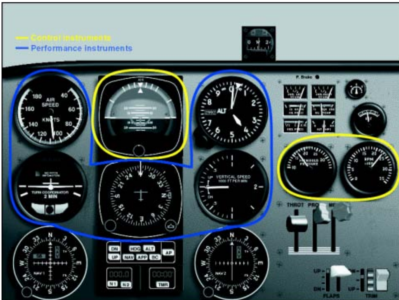
Figure 4-1. Control/Performance cross-check method.
