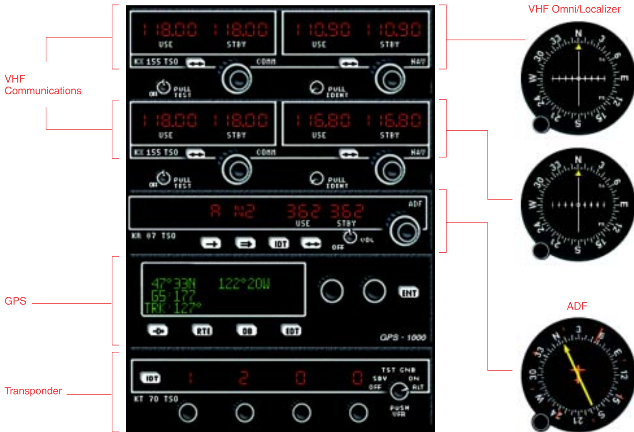
Figure 9-1. Typical NAV/COM installation.
