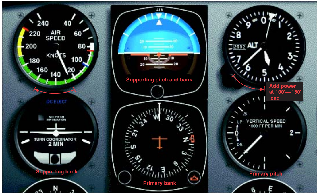
Figure 5-31. Level-off airspeed higher than descent airspeed.
