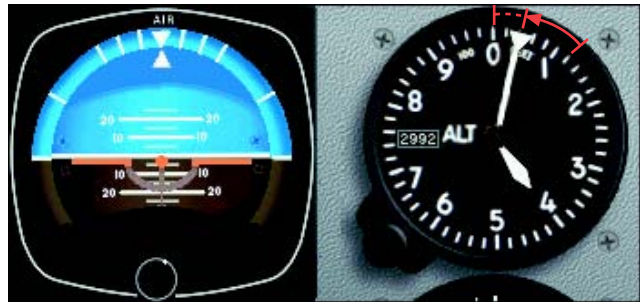
Figure 5-8. Pitch correction following altitude increase—lower nose to correct altitude error.
