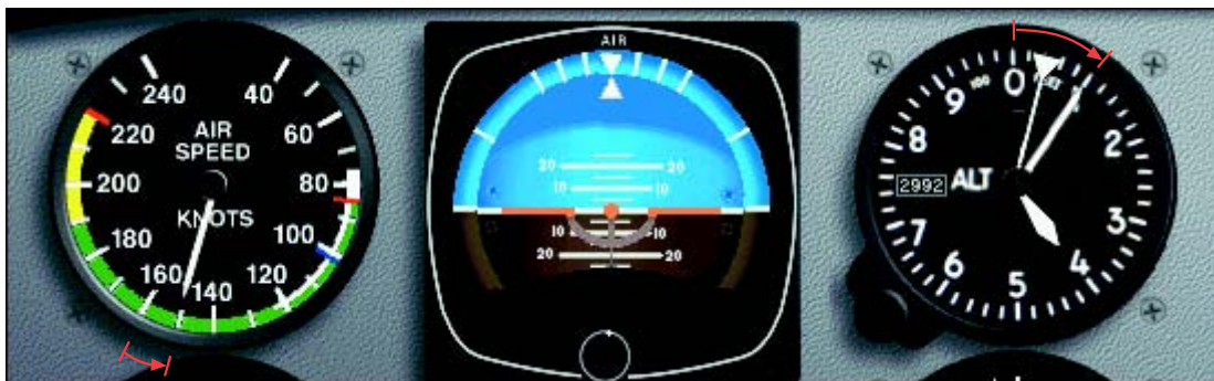
Figure 5-20. Airspeed low and altitude high (lower pitch).
