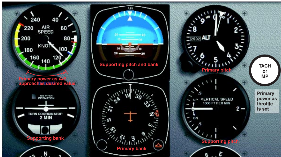
Figure 5-23. Straight-and-level flight (airspeed decreasing).
