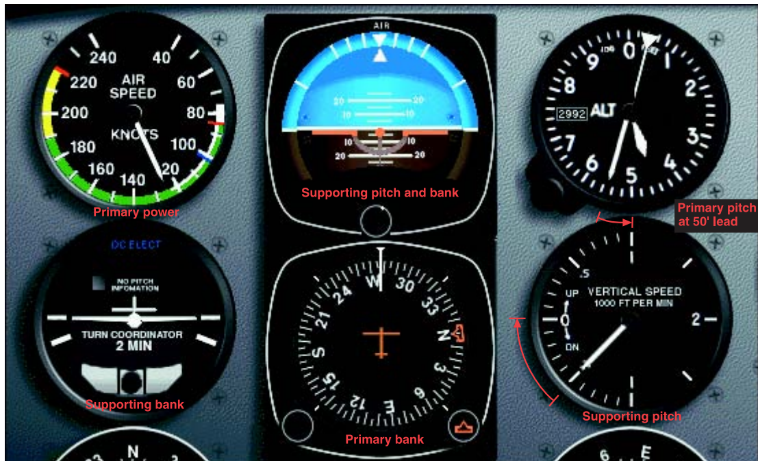
Figure 5-32. Level-off at descent airspeed.
