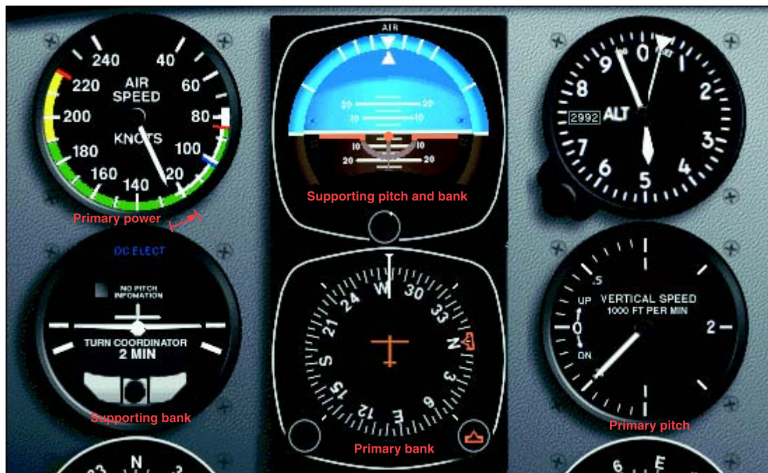
Figure 5-30. Constant airspeed descent, airspeed high—reduce power.
