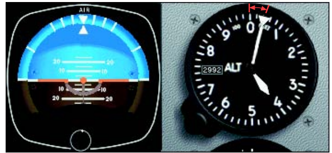
Figure 5-9. Altitude error, less than 100 feet.
