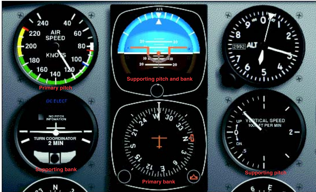
Figure 5-26. Stabilized climb at constant airspeed.
