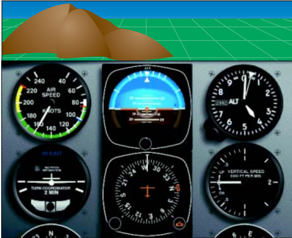
Figure 5-3. Pitch attitude and airspeed in level flight, normal cruise speed.
